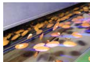
The IXUS BULK's x-ray sorter sorts almonds for production.
