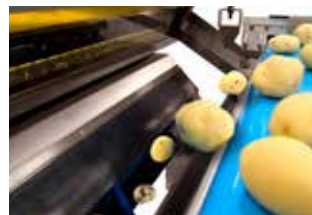
The TITAN II's NIR optical sensors sort a potato product for shipment.
